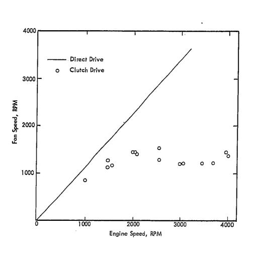
Figure 35. Speed of Clutch Fan and Direct Drive Fan, Ford F-150.
