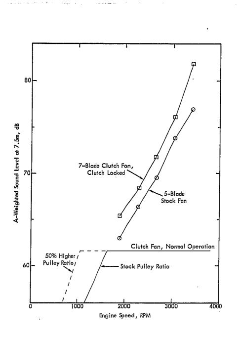
Figure 36. Noise Levels of Stock Fan and Clutch Fan, Ford F-150.
