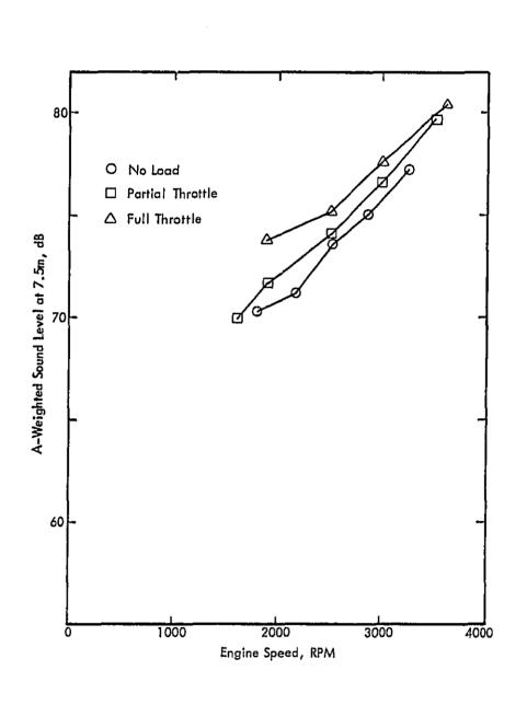
Figure 17. Sideline Noise Characteristics of Oldsmobile Diesel.
