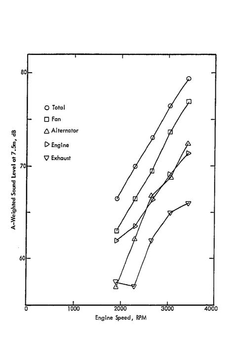
Figure 19. Noise Source Components at No Load, Ford F-150.
